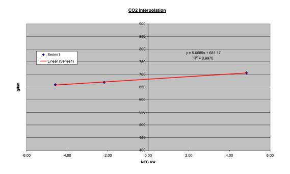
The bus was found to have a  $CO_2$  output when corrected for zero NEC of 681.17 g/km.
